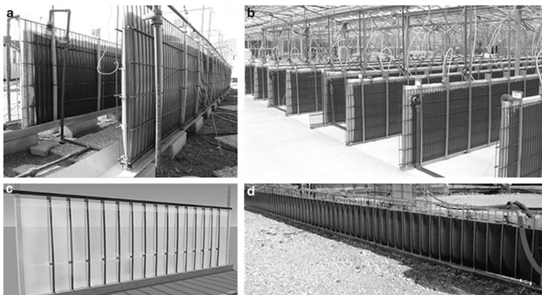
Fig. 7.2 Green Wall Panel (GWP) photobioreactors developed at the University of Florence (2004–2009) and commercialized by F&M S.r.l. (a) 20-m-long GWP prototype; (b) GWP pilot-scale plant (5,000 L) in
