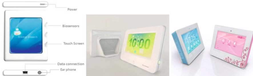
Fig. 10.11 Hardware prototype of Sleep Coach
