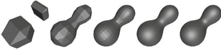
Fig. 12 Two blobs [14] represented, from left to right , with a higher level of detail
