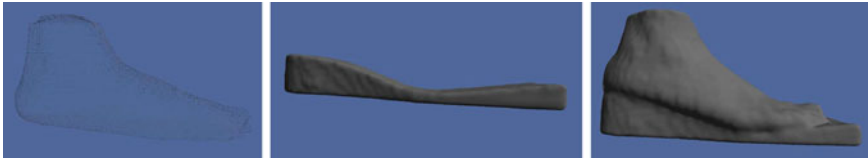
Fig. 2 Basic elements needed for simulation of a foot deformation. Left cloud of points of the scanned foot. Center scanned platform shoe. Right scanned of the foot and platform together
