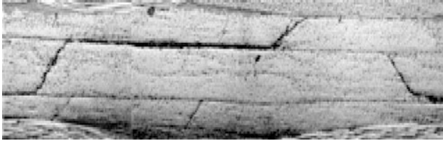
Fig. 8 Micrograph showing delamination starting from cracks in resin pocket and connected by intralaminar cracks in FT laminates (Table 1), t = 2 mm
