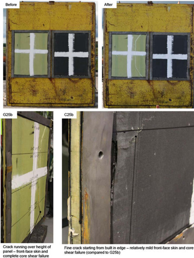
Fig. 14 (a) Before and after images taken of the front face view of G3 and C1 after being subject to a charge of 100 kg TNT equivalent at stand-off of 14 m. (b) Images featuring the damage sustained by G3 and C1 after being blasted
