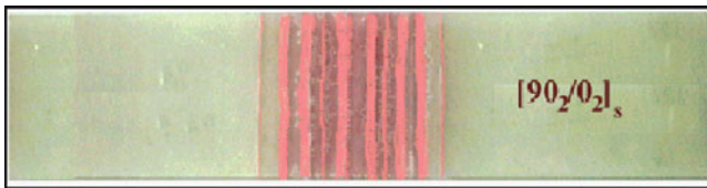
Fig. 22 Transverse stripes delamination (in red) of [90_2/0_4/90_2] (top view)
