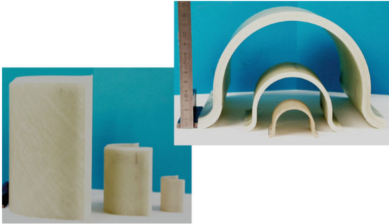
Fig. 5 Structures featuring three different scales (1; 1/2; 1/4)
