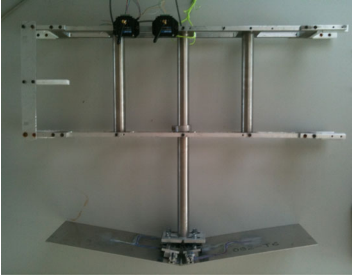
Fig. 4 Picture of the sledge with an aluminum wedge mounted on it
