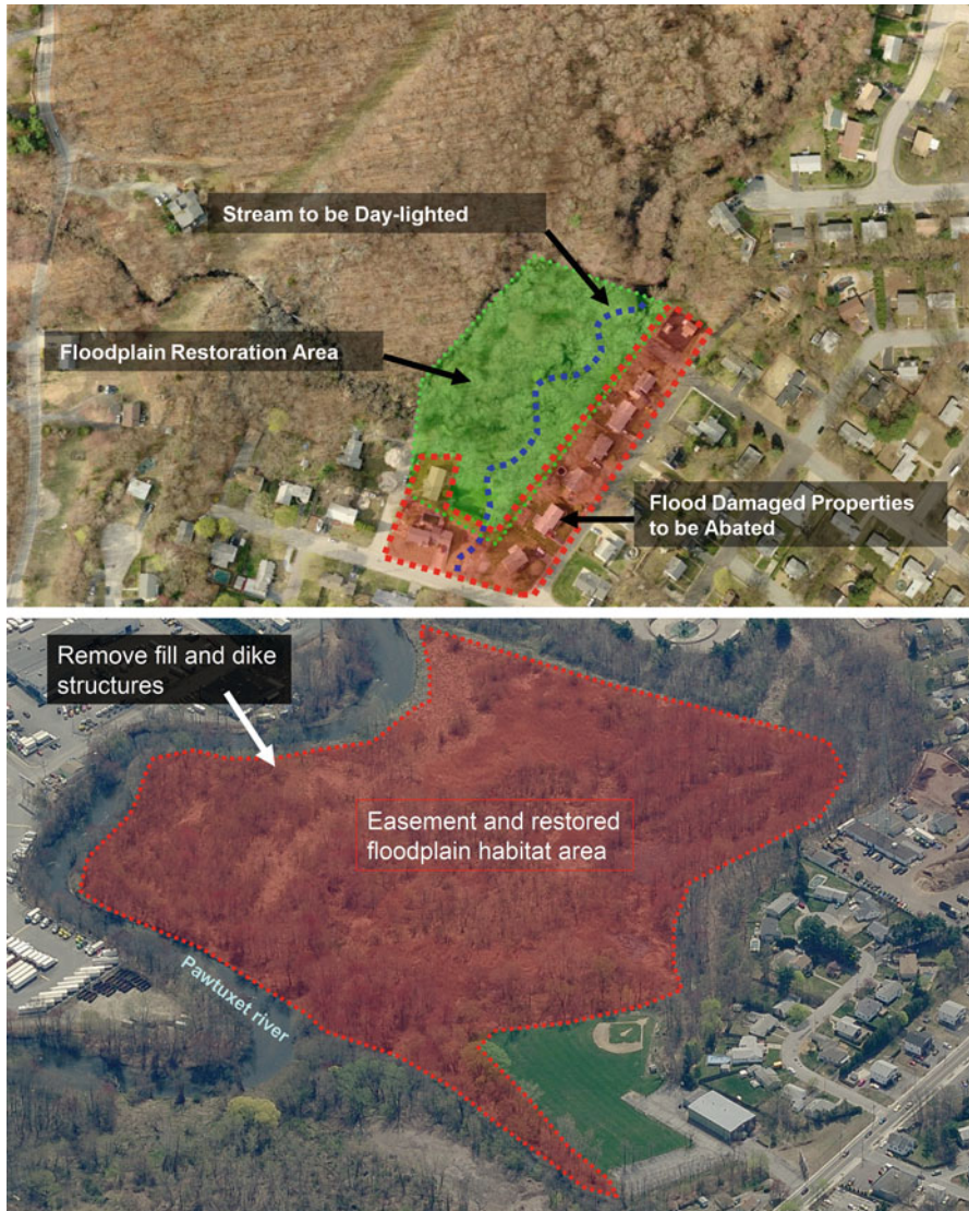
Fig. 4.5 Rhode Island NRCS floodplain restoration projects. (a) Meshanticut River Headwater (Janet Drive) floodplain in West Warwick- removal of a culvert and creation of a new, open stream channel. (b) Pawtuxet and Pocasset River confluence floodplain in Cranston- removal of a dike and floodplain fill to restore connectivity (Photos courtesy of USDA Natural Resources Conservation Service, Rhode Island (2011))
