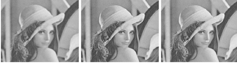
Fig. 12.6 “Lena”. Left : A blurred noised image, t = 2.5 , noise STD = 10, PSNR = 24.79. Center : An image restored by GTA, PSNR = 28.22. Right : An image restored by BBA, PSNR = 28.47, spline wavelet packets of the fourth order from 4 levels were used
