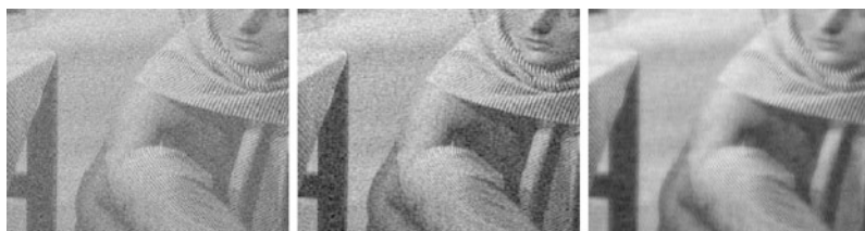
Fig. 12.4 “Barbara”. Left : A noised image, STD = 25 , PSNR = 20.17 . Center : An image restored by GTA, PSNR = 24.12 . Right : An image restored by BBA, PSNR = 25.77 , spline wavelet packets of the fourth order from 4 levels were used
