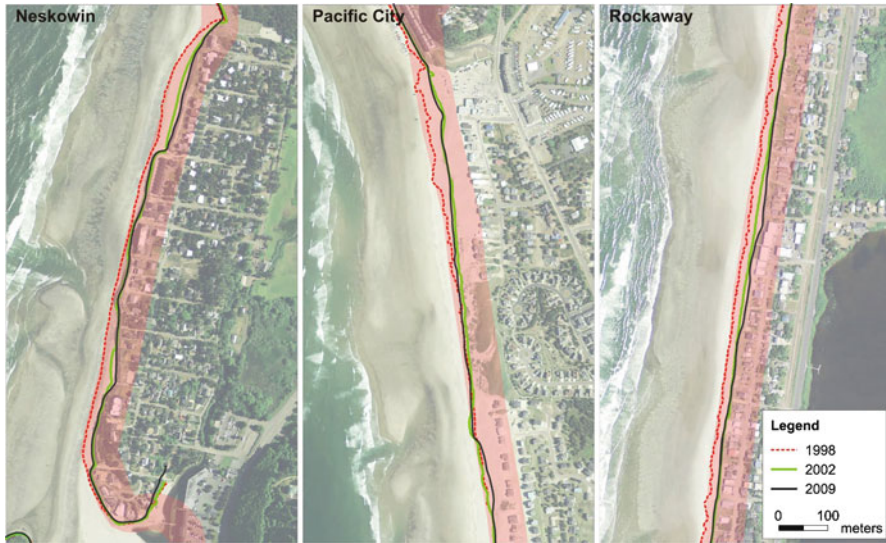
Fig. 21.47 Examples of high-risk erosion hazard zones in foredunes along the Oregon coast. Lines included in the figure indicate the positions of the dune toe (~6 m elevation) in various years, while the red areas represent the high-risk hazard zones (After Allan and Priest (2001))
