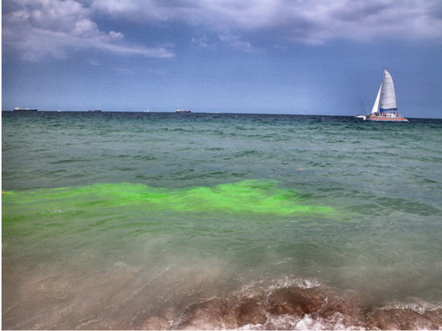
Fig. 26.13 Fluorescent dye, which is non-toxic, biodegradable, and NSF-approved as safe in drinking water ( www.hazard.com/msds ) in the form of a dye ball can be safely thrown from shore; it quickly dissolves in the water to form a plume that moves with any currents present (Source: S. P. Leatherman)
