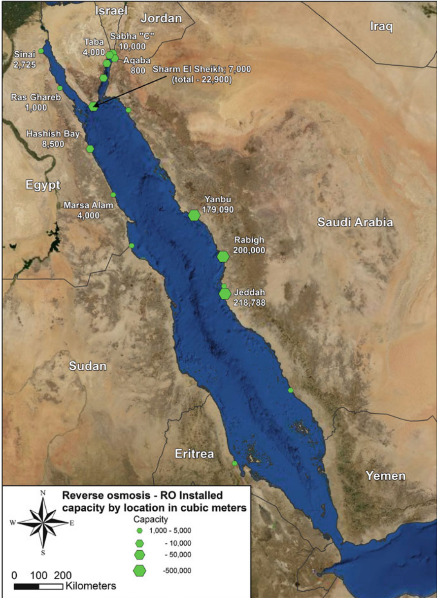
Fig. 12.2 Several RO desalination plants on Red Sea coast (El-Sadek 2010; Lattemann and Höpner 2008; Mohsen 2007; Khalil 2004; Semiat 2001) (Source of background: Esri, i-cubed, USDA, USGS, AEX, GeoEye, Getmapping, Aerogrid, IGN, IGP, and the GIS User Community)
