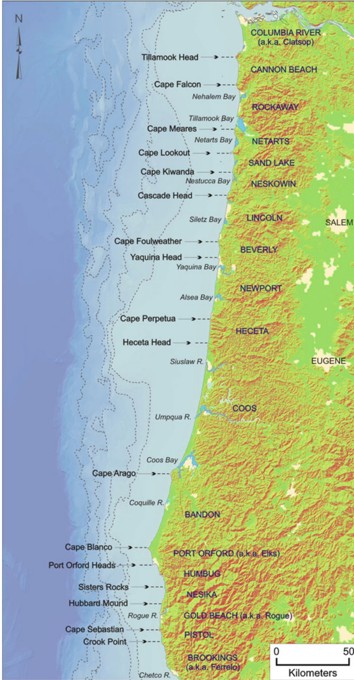
Fig. 21.5 The major headlands defining the principal littoral cells along the Oregon coast
