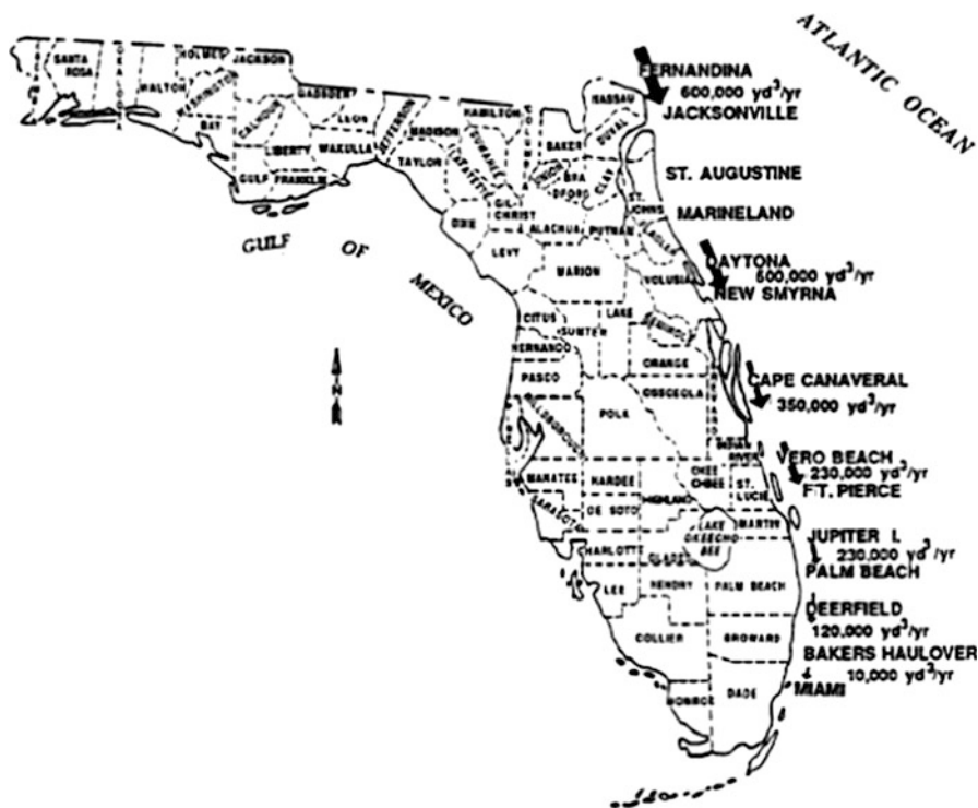
Fig. 13.19 Estimated net longshore sediment transport along Florida's east coast. Transport quantities in cubic yards per year
