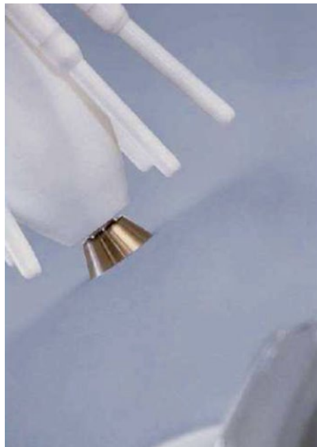
Fig. 2.30 Multi feed bell seven feed tubes are installed in the pipe inside of the bell
