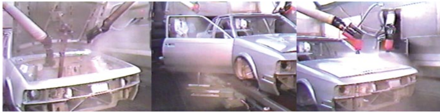
Fig. 2.44 Photo pictures of modular painting system in GM
