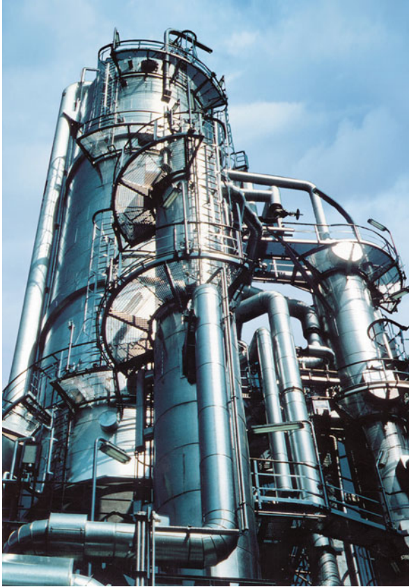
Fig. 2.11 In the distillation plant in the refinery, crude oil is further processed, e.g. into petrol, http://www.deutschebp.de/liveassets/bp_internet/germany/STAGING/home_assets/images/raffinerie_verarbeitung/A8_Destillation_HighRes.jpg (retrieved April 8th 2013)
