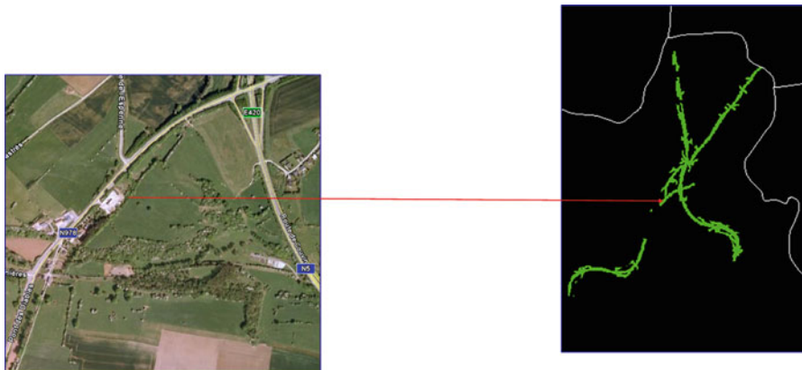
Fig. 6.10 Stretch of road resulting from the reclassification of the final map
