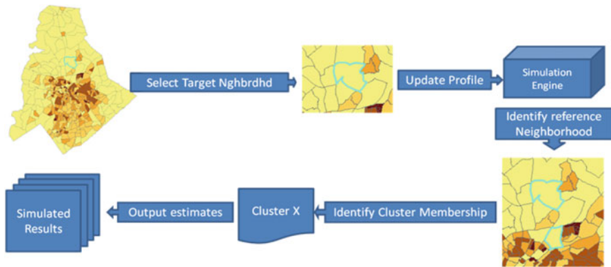
Fig. 11.1 Simulation Algorithm: from selecting a target neighborhood, updating its profile, identifying a reference neighborhood and cluster membership, to outputting simulated results
