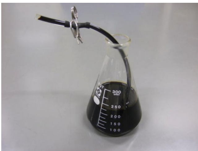
Photo 4 Absorbent solution ready for injection into the syringe
