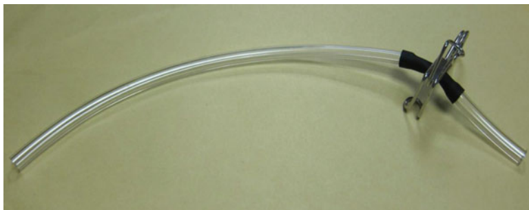
Photo 3 A prepared tube for introduction of absorption solution into the syringe
