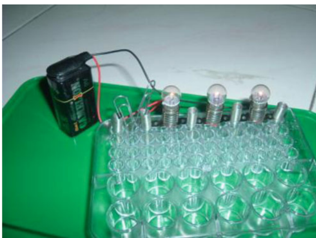
Fig. 3 Parallel circuit in microscale set-up
