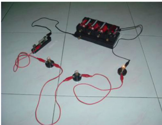
Fig. 2 Parallel circuit in traditional set-up
