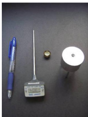
Size of aluminum block calorimeter and digital thermometer
