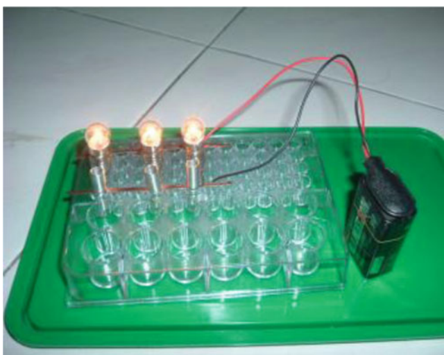
Fig. 5 Series circuit in microscale set-up
