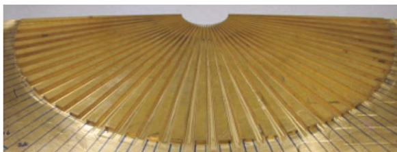
Fig. 7.9 The acoustic hyperlens sample. The lens is made of 36 brass fins in air (running from radius 2.7 to 21.8 cm in the radial direction). The fins, spanning 180 degrees, are sitting on a brass substrate. The cover sheet has been removed to expose the microstructure for this view. Reproduced from [34] with permission of Nature Publishing Group
