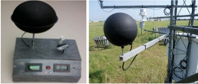
Fig. 26.3 Black Globe Temperature Sensor used in preliminary tests ( left ). Black Globe Temperature Sensor for Heat Stress used to verify equations at the Oklahoma Mesonet test facility in Norman Oklahoma ( right )
