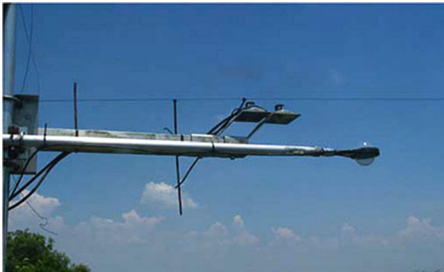
Fig. 2.20 A Q7.1 net radiometer from a weather station in south Florida (Photograph provided by South Florida Water Management District)
