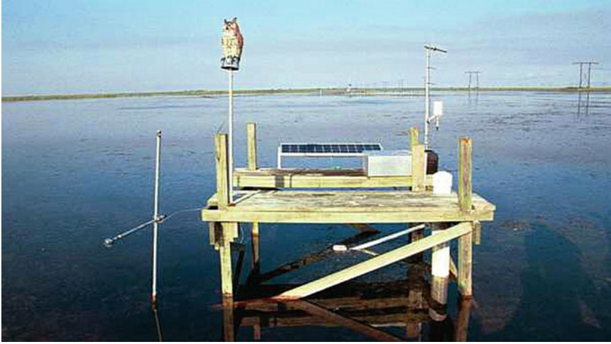
Fig. 3.8 Bowen ratio instrumentation site in the Everglades Nutrient Removal Project (German 2000; U.S. Geological Survey)
