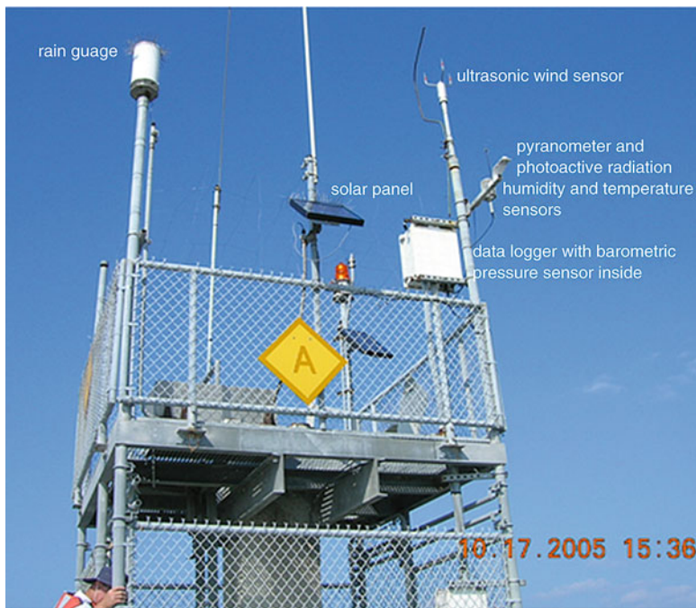
Fig. 2.1 A weather station in Lake Okeechobee, south Florida (Photograph provided by South Florida Water Management District)
