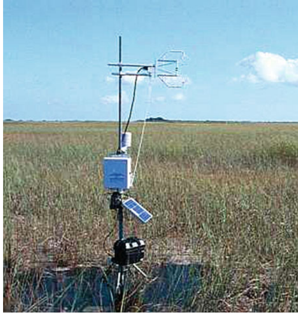
Fig. 3.6 Eddy correlation instrumentation in the Everglades (German 2000; U.S. Geological Survey)
