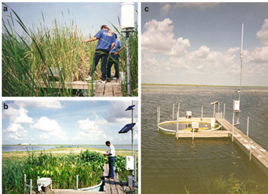
Fig. 3.4 (a) Cattails, (b) mixed marsh, and (c) open water lysimeters (Photograph provided by South Florida Water Management District)
