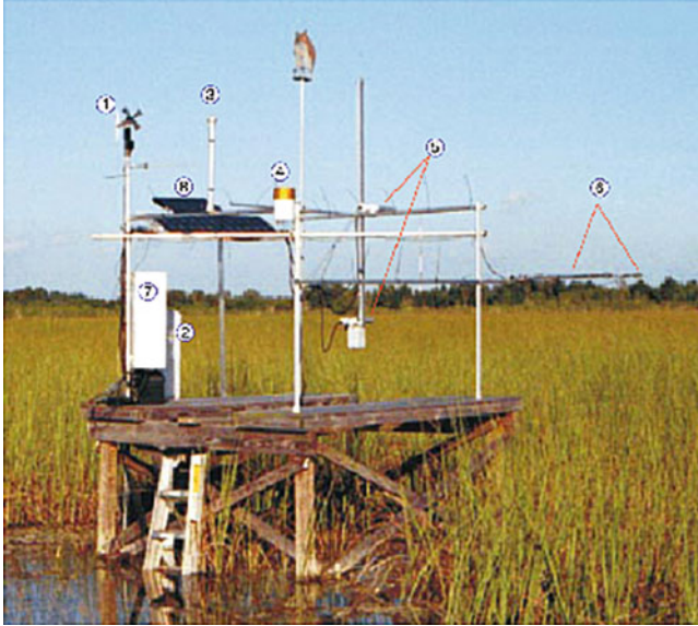
Fig. 3.7 Bowen ratio instrumentation site in the Everglades (German 2000; U.S. Geological Survey; Abtew 2005)
