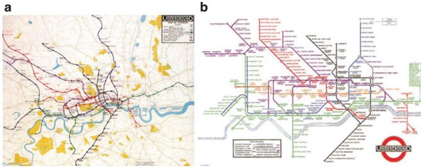
Fig. 8.1 Two versions of the London underground map: (a) a geometric map and (b) a topological map
