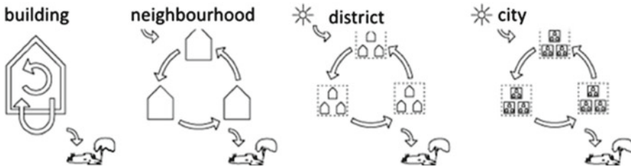
Fig. 9.5 Reuse of waste flows and upscaling from building to city level
