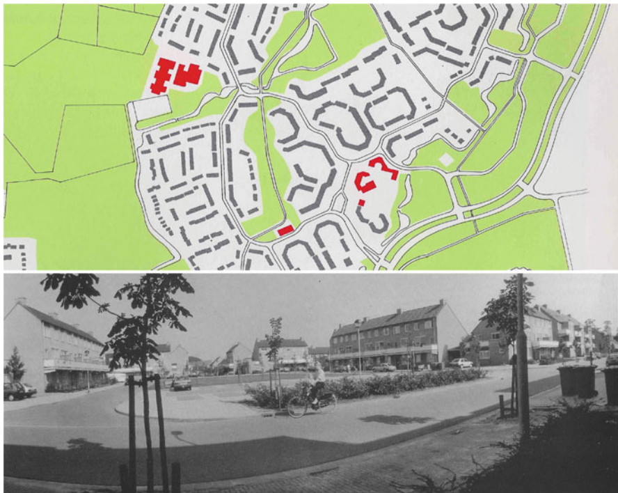
Fig. 2.3 Haagse Beemden: section of the lay out (De Boer and Lambert 1987) and typical view of a ‘woonerf’ (a car-free, dead-end street with street furniture, playgrounds and priority for pedestrians, cyclists and playing children) (Otten and Dijkstra 1989)
