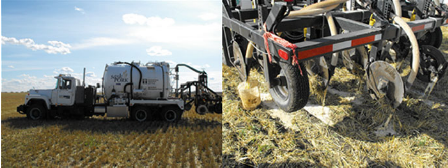
Fig. 2 Liquid manure application equipment ( left ) used during thin stillage injection ( right ) in a field trial in east-central Saskatchewan, Canada
