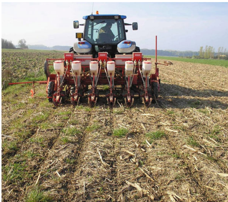
Photo 3 Direct seed drilling over the residue of previous crop under no-tillage system. Layer of crop residues on the surface conserve soil moisture and nutrient and also reduce soil erosion
