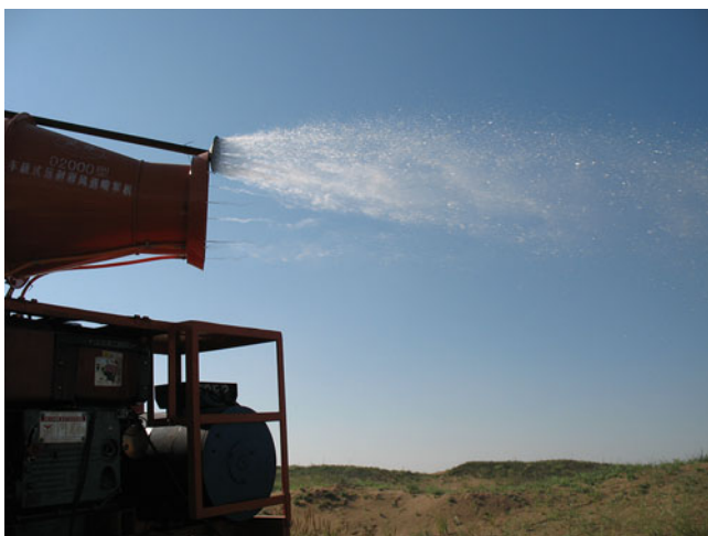
Fig. 12.3 Truck equipped with an improved sprinkler head spraying an algal suspension up to a distance of 50 m. Qubqi (Hobq) Desert, Dalateqi, Inner Mongolia, in August 2007
