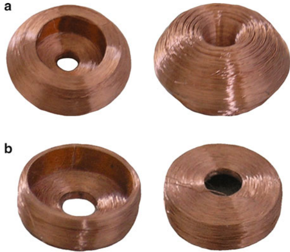
Fig. 6.13 Without an appreciable loss in the output power the optimal coil topology can be idealized to a cap like shape
