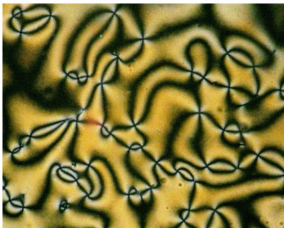
Fig. 4.3 Schlieren textures of SmC phase of the symmetric nonyl derivative 1 (bromide salt) at 90°C with only four-brush defects (Reproduced from Ref. [31] with kind permission of © Elsevier)
