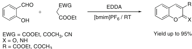
Scheme 17.11 Knoevenagel condensation between aldehydes or ketones using [bmim]PF 6
