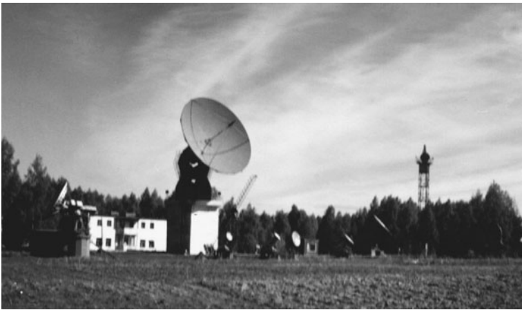
Fig. 2.7 Seven-metre radio telescope and tower with the black disk (Staraya Pustyn' station)
