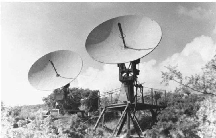
Fig. 1.9 Interferometer formed of two radio telescopes. The diameters of these parabolic dishes are 4 m. Observations at decimetre and centimetre wavelengths were carried out on this interferometer
