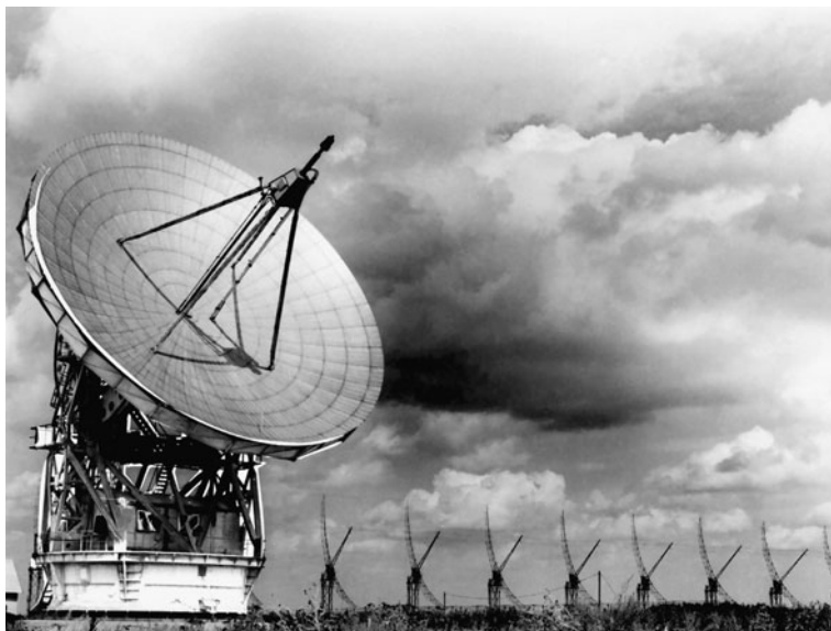
Fig. 1.12 The 22-m radio telescope of FIAN. The first complex of radiometers (0.8 and 3.2 cm) is at the focus of the parabolic surface
