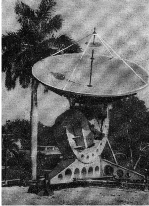
Fig. 4.3 Three-metre GAO antenna with an equatorial mount installed in Cuba
