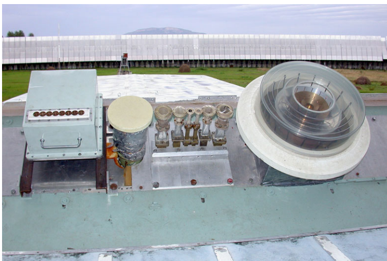
Fig. 5.4 Primary feeds on the focal line of the parabolic cylinder
