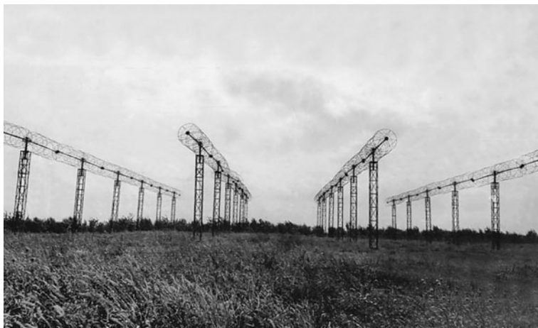
Fig. 8.1 Antenna arrays of the second version of the ID-1 interferometer
