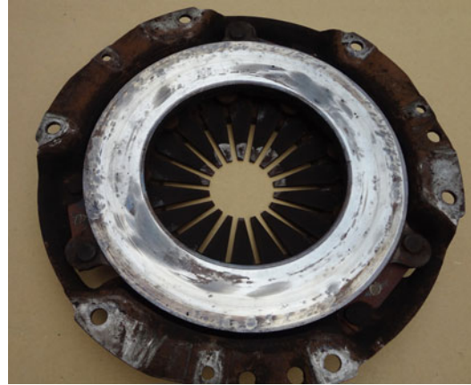
Clutches, Hot Spotting Behavior, Fig. 3 Hot spots on the surface of cast iron plate of an automotive dry clutch
