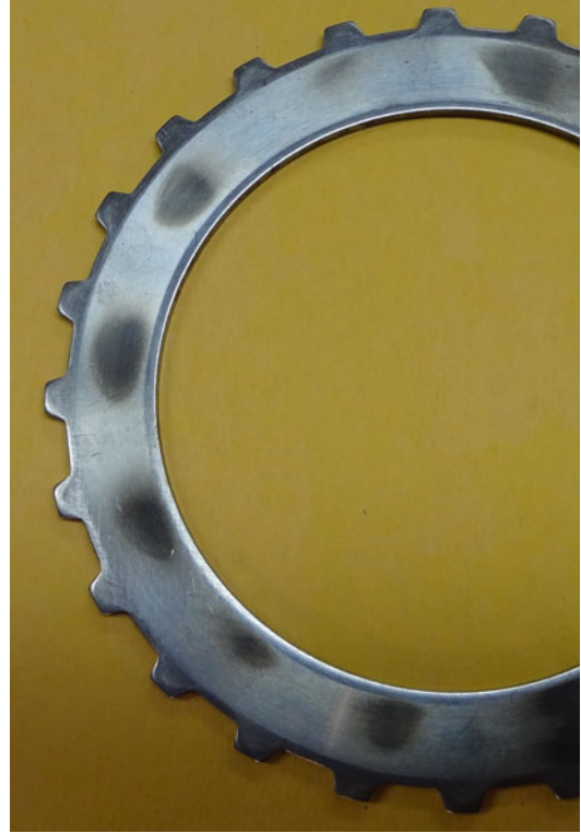
Clutches, Hot Spotting Behavior, Fig. 1 Hot spots on the surface of steel disk of a wet clutch produced after single clutch engagement
