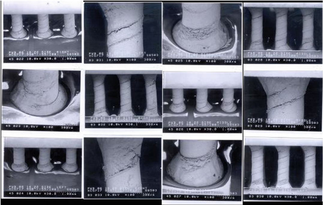
Column Grid Array Assembly Under Thermal Cycling Stress, Fig. 5 SEM photomicrographs of CGA 717 I/O assembly at 950 thermal cycles ( -55\text{ }^{\circ}\text{C}/100\text{ }^{\circ}\text{C} ) showing signs of microcracking
