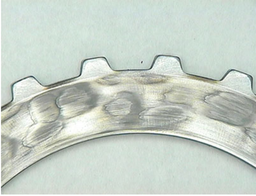
Clutches, Hot Spotting Behavior, Fig. 2 Hot spots on the surface of steel disk of a wet clutch after multiple engagements
