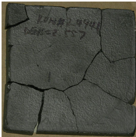
Control of Thermal Residual Stresses, Fig. 4 Possible effect of uncontrolled thermal stresses
