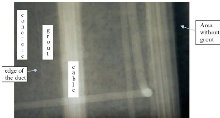
Fig. 7.4 Example of radiogram – sounding of an internal tendon [AFGC-B7, 2005]
