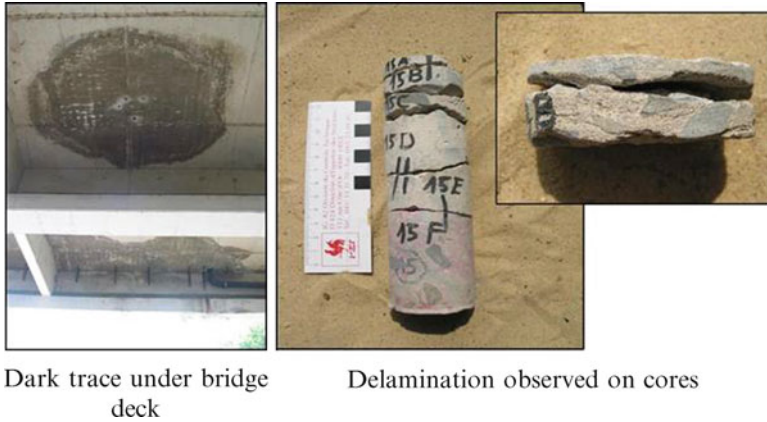
Fig. 5.18 Visual detection and destructive study of interfaces on Lommersweiler bridge, Belgium (Gilles, 2004)
