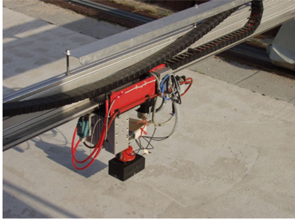
Fig. 2.11 2D scanner working with linear drives and a pneumatic system to press the point contact transducers without coupling agent (BAM) [Beutel et al., 2006]
