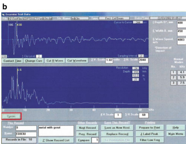
Fig. 6.10b) Result of impact-echo test over a grouted tendon duct [Forde, 2006]
