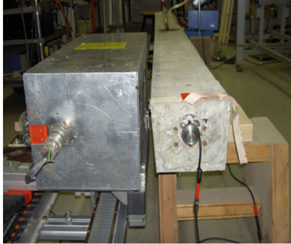
Fig. 7.23 Laboratory prestressed beam for detecting a wire failure by magnetic flux leakage method [Sawade, 2007]
