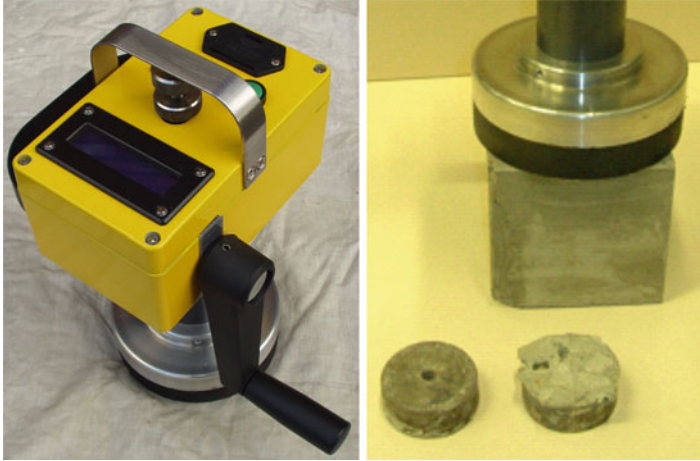
Fig. 3.5 Portable Pull-off Tester (left), circular steel probe (right)
