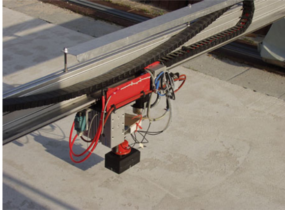
Fig. 6.24 2D scanner working with linear drives and a pneumatic system to press the point contact transducers without coupling agent (at BAM Berlin)
