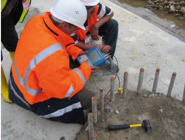
Fig. 4.22 Performing the Impulse response method
