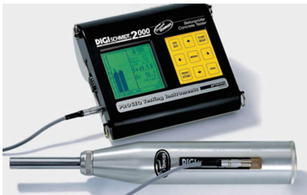
Fig. 2.3 Typical digital Rebound Hammer
