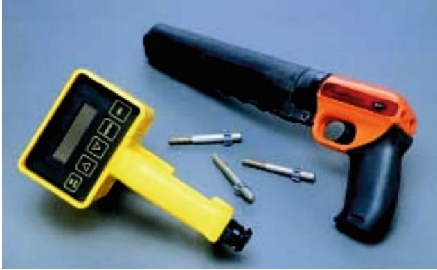
Fig. 3.1 Penetration resistance probes and associated equipment
