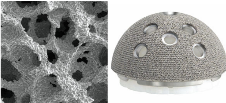
Fig. 3.6 High-power photomicrograph of Tritanium metallic coating and its application to a primary total hip acetabular component. (Courtesy of Stryker, Mahwah, NJ)
