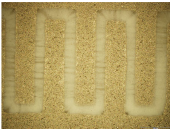
Fig. 5.17 Optical image of a thin film of \text{TiO}_2 deposited on alumina substrate with interdigitated electrodes. The device serves as an electrochemical (bio) sensor
