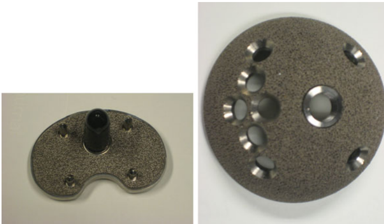
Fig. 3.5 Titanium foam coated tibial baseplate and acetabular components currently available for clinical use
