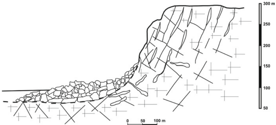
Fig. 13.7 Draft profile of the Joc rockfall (Sunarić 1976)
