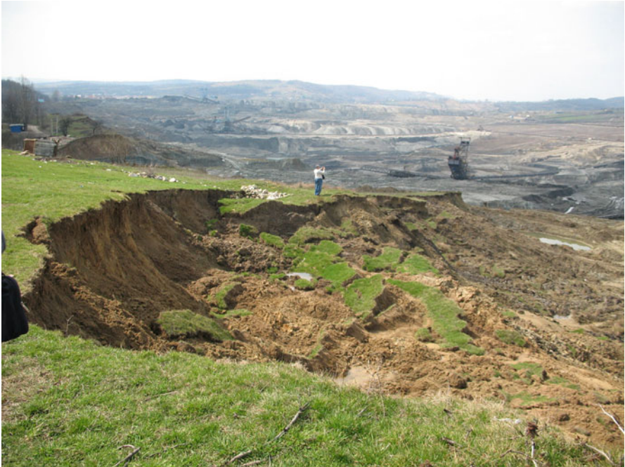
Fig. 10.3 Deep-seated slump at the margin of a coal quarry, Berbești (Getic Subcarpathians) (Photo: Marta Jurcescu)
