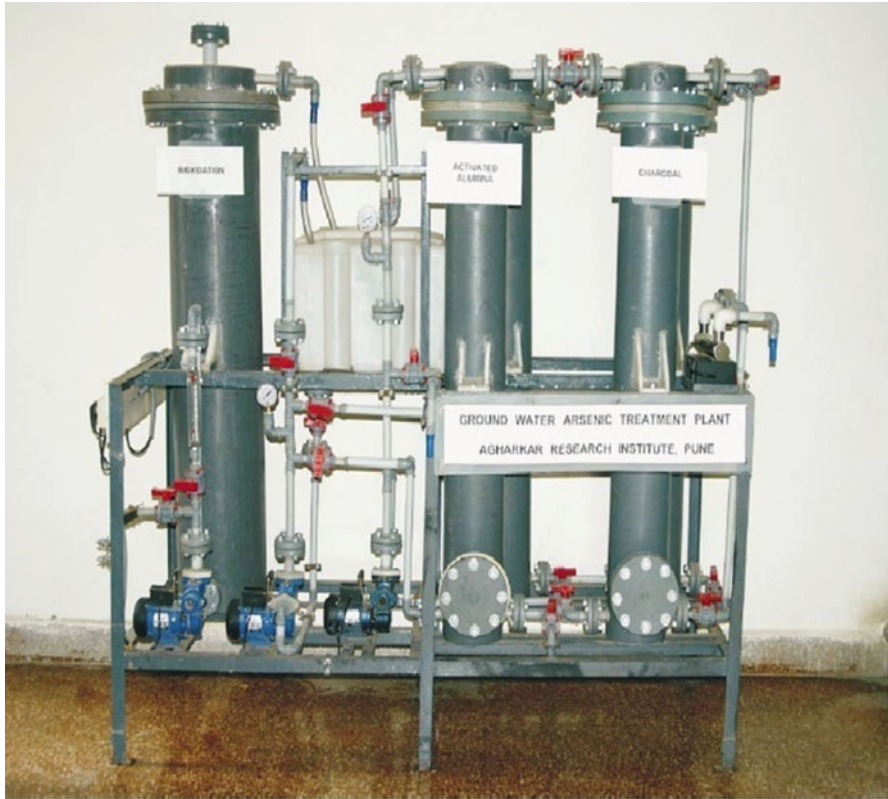
Fig. 22.4 Integrated field scale system working on bio-oxidation alumina adsorption technology installed in arsenic affected areas of Rajnandgaon District, Chhattisgarh
