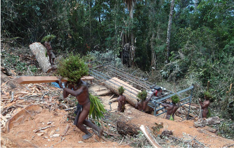
Fig. 11.8 Kgwán community members establishing a portable sawmill, near Gembogl, Papua New Guinea Highlands (Photo courtesy Julian Fox)
