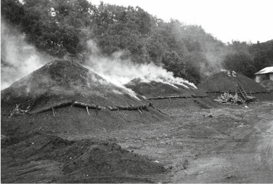
Fig. 6.4 Charcoal making in Pindos Mountains, northwest Greece. From the right : kilns in the second, sixth and tenth day of burning. June 2001 (Photo: Eirini Saratsi)
