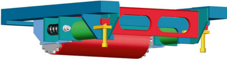
Fig. 17.1 Sketch of the FRP prestressing machine, seen from the beam midspan side
