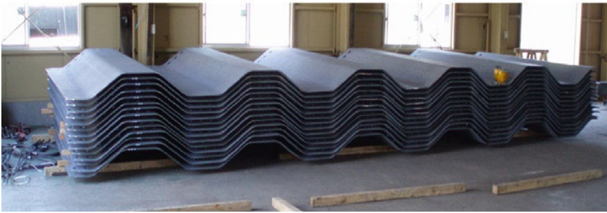
Fig. 22.17 A sophisticated press and fabricated corrugated webs
