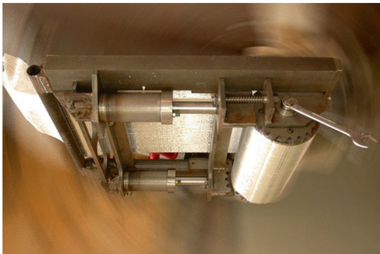
Fig. 17.4 An FRP prestressing machine prototype with GFRP fabric mounted for tests
