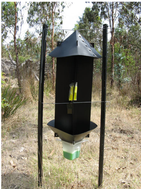
Fig. 12.1 Intercept ® trap used for Sirex detection, showing pinene lure (yellow) and Ethylene glycol preservative (green)
