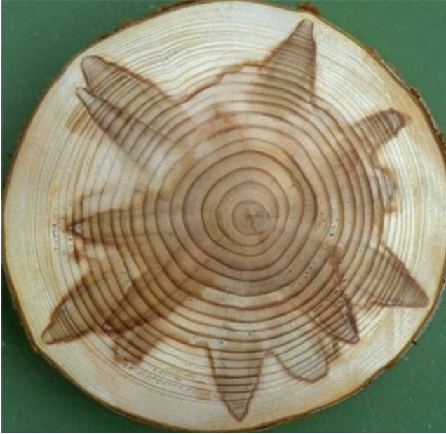
Fig. 7.1 Wood discoloration in a cross section of Cryptomeria japonica stem caused by Urocerus japonicus and Amylostereum laevigatum
