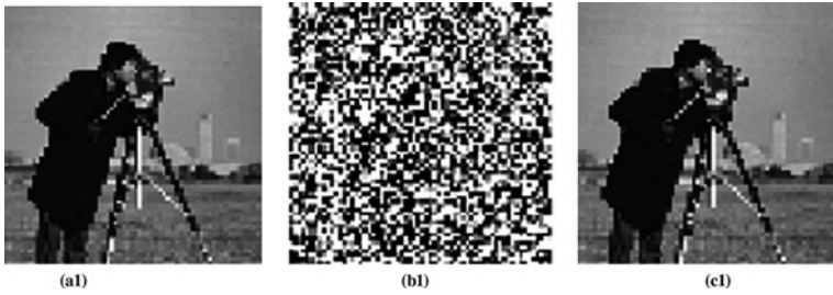
Fig. 60.2 Scrambling on the gray image and recovery them a1 original cameraman image b1 scrambled cameraman image c1 restored cameraman image (PSNR = 50.9343 dB)
