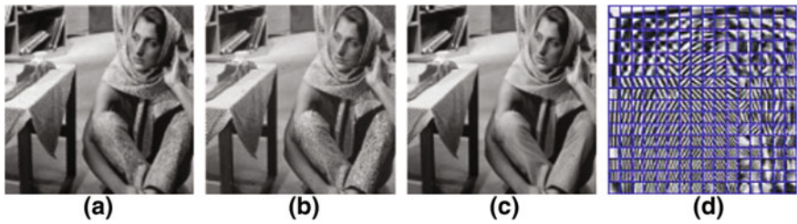
Fig. 58.2 Denoised results by a L1-TV b L1-SKR and c-d AL-ADM-DL and the learned dictionary. p = 20\%
