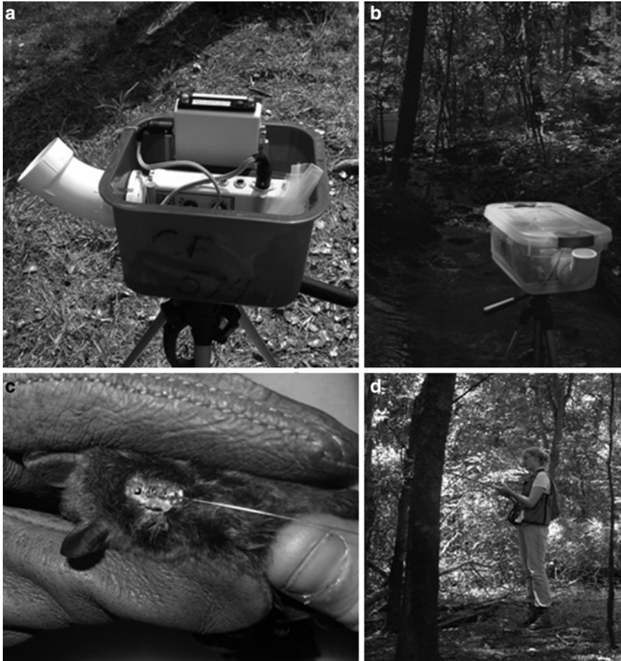
Fig. 10.2 Techniques used to determine use of different habitat types by bats. (a) An Anabat II bat detector system, (b) the Anabat II system deployed in the field, (c) an Indiana bat with a radio transmitter, and (d) tracking a bat with an antenna and receiver
