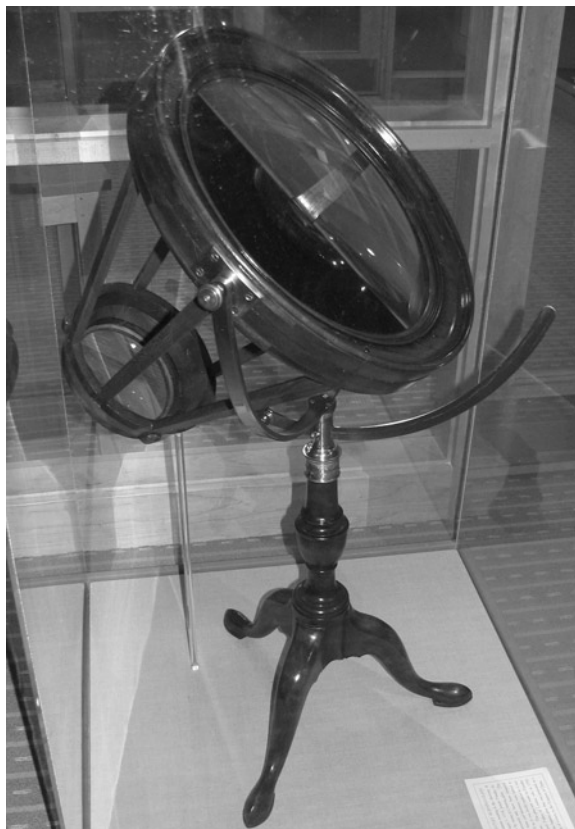
Fig. 30.7. A compound burning-glass used by Joseph Priestley. The lenses are 16 and 7 in. in diameter, 16 in. apart. The glass is housed in the Archives and Special Collections, Dickinson College, Carlisle, Pennsylvania (Photo by the author).
