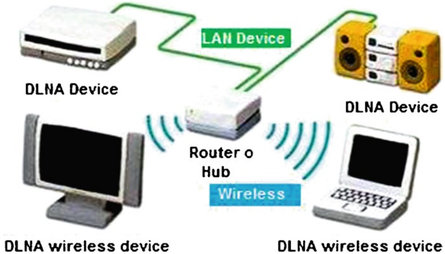
Fig. 1.26 Interoperability between two devices using DLNA
