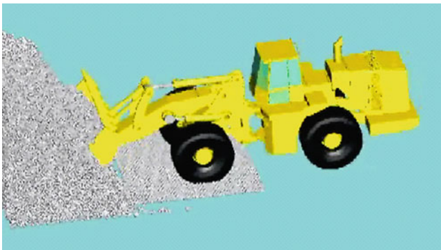
Fig. 3 Medium wheel loader bucket loading – dumping operation (granular material) using Rocks3D TD
