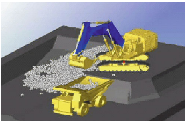
Fig. 1 Hydraulic excavator bucket loading – dumping operation (granular material) using Rocks3D TD
