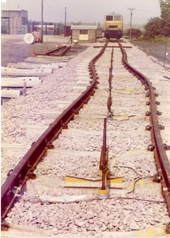
Figure 1. Buckling of linear structures (railroad tracks) into curves in a plane, due to thermal expansion, which generates compressive forces on the rails (Coxon, 1979; Reproduced with kind permission of the photographer, Dave Coxon). This is an example of buckling from one to two dimensions. The rails buckle the same way because they are coupled via the perpendicular ties.
