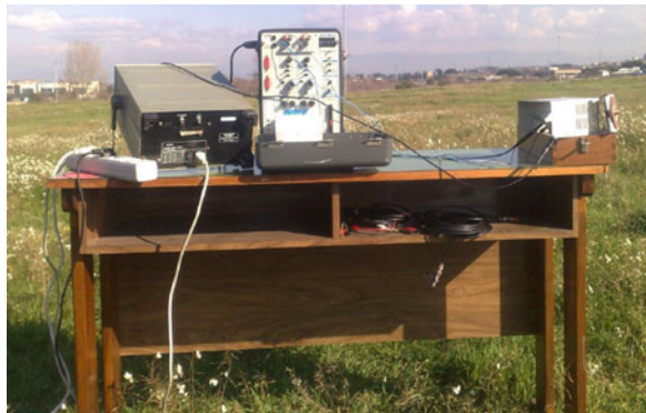
Fig. 26.4 Experimental set up for the preliminary experiments in a partially cloudy day. Changes of the electric field (from 20 to 30 V/m at sunset in a sunny day), up to 800 V/m (during clouds displacement) have been detected
