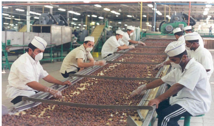
Fig. 32.1 An inspection belt for dates grading for size and quality prior to bulk packing (Source: Dates Processing Factory, Ministry of Agriculture, Al-Hassa, Saudi Arabia, 2002)
