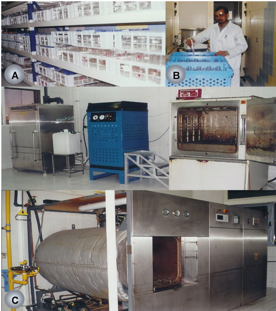
Fig. 8.5 Tissue culture facilities. (a) Media storage room, (b) Media filling area, (c) Autoclave rooms
