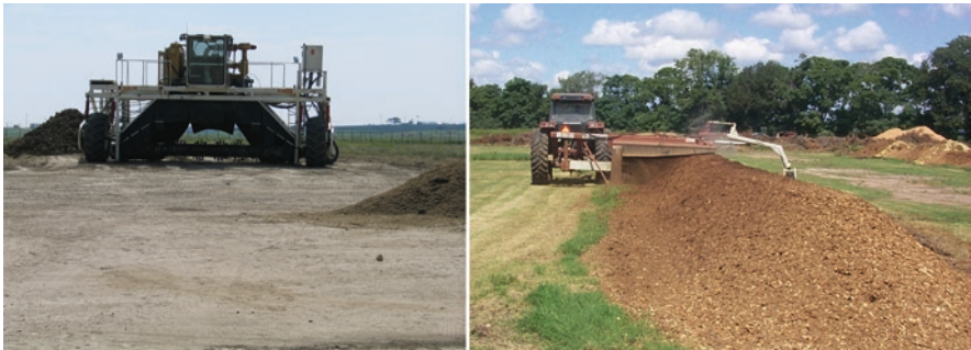
Fig. 3 Windrow/biopile turning machines in Texas, USA (Photos courtesy of Saqib Mukhtar)
