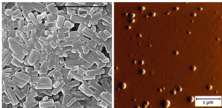
**Fig. 1** Crystalline nanocrystals with cuboid shape (*left*, Courtesy by Böhm (1999), Modified) and nanoMorph amorphous drug nanoparticles of spherical shape due to lack of ordered crystal structure (*right*, Courtesy by Soliqs, Ludwigshafen, Germany)
