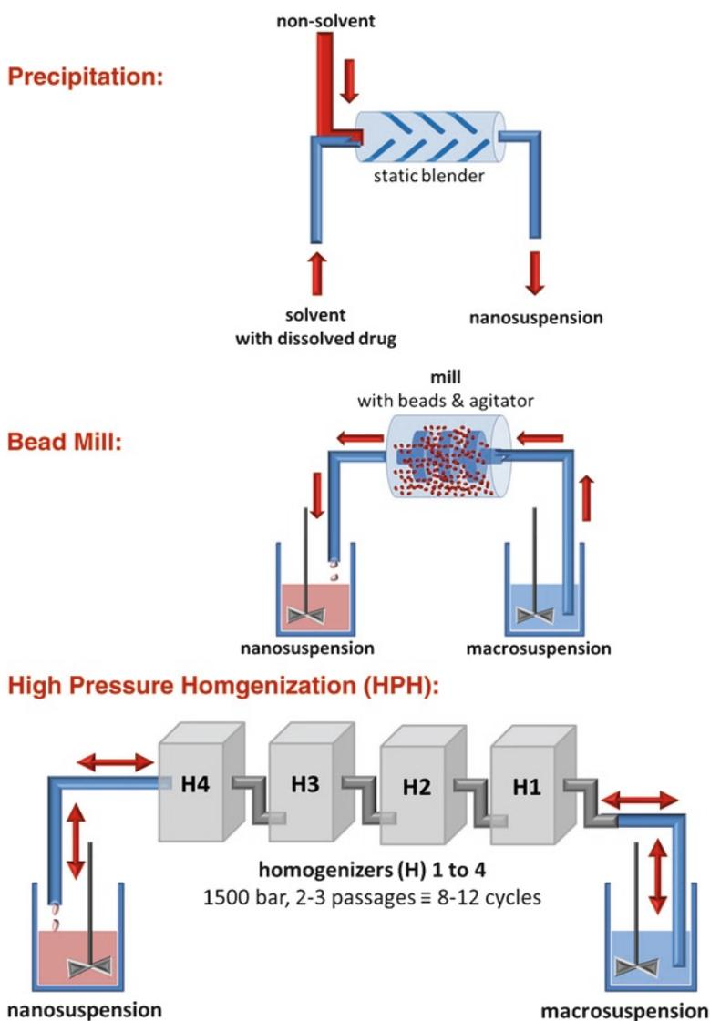
**Fig. 2** Large scale production of nanocrystals (explanations cf. text): *upper* – solvent with drug and non solvent are mixed in a static blender; *middle* – macrosuspension is passed multiply from two containers through a bead mill; *lower* – four homogenizers in line for nanocrystal production, one pass is equivalent to four homogenization cycles
