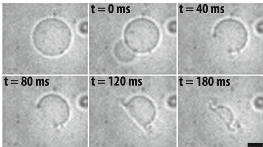
**Fig. 14** Snapshots of an ePBD-iPAzo polymersome bursting under UV illumination. Bright-field images were taken using a high-speed digital camera. The first image shows the vesicle prior to illumination. Time  $t=0$  corresponds to pore nucleation. The expulsion of sucrose solution is visible as the pore nucleated. The other images correspond to pore growth and clearly show outward spirals (scale bar =  $5 \mu\text{m}$ )
