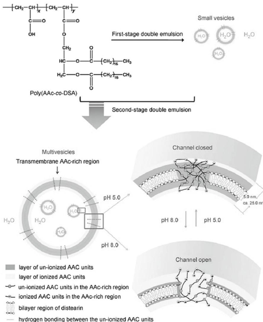
**Fig. 3** Illustration of multi-vesicular assemblies produced via a two-stage double emulsion of poly(AAc-co-DSA). The resulting vesicles are equipped with pH-responsive transmembrane channels. (Reproduced from ref. Chiu et al. 2008)
