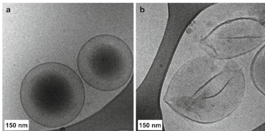
**Fig. 13** Cryo-transmission electron micrograph of the polymersomes formed in water by the PEG-*b*-azodendron block copolymer **PEG45-AZO16** (a) before and (b) after illumination with 360 nm unpolarized light (150 mW/cm<sup>2</sup>) for 35 min
