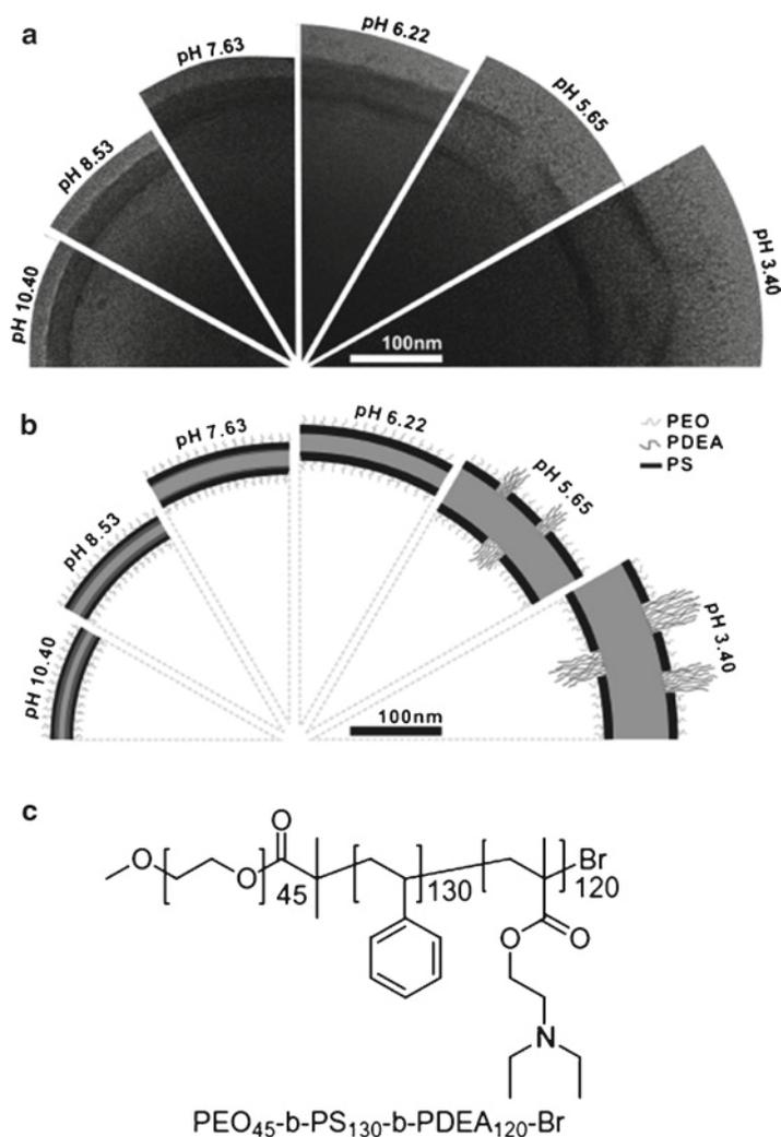
**Fig. 4** (a) cryo-TEM images of vesicle wall structures at pH 10.4, 8.53, 7.63, 6.22, 5.65, and 3.40, respectively; (b) schematic illustrations of the three-layered wall structures at corresponding pH values; (c) the chemical structure of the triblock copolymer used to form the breathing polymersomes. (Reproduced from ref Yu et al. 2009)
