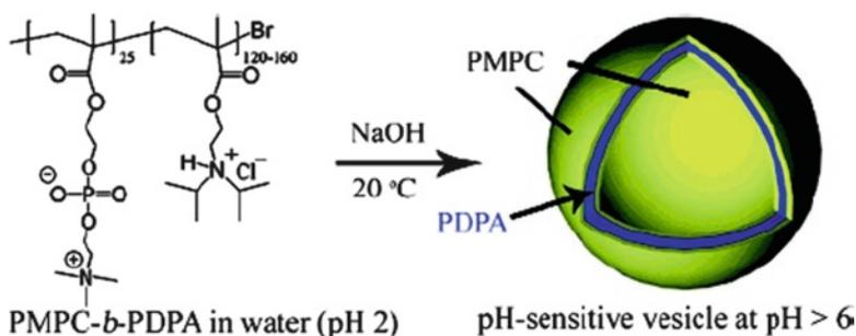
**Fig. 5** Formation of PMPC-*b*-PDPA block copolymer vesicles. (Reproduced from ref. Du et al. 2005)
