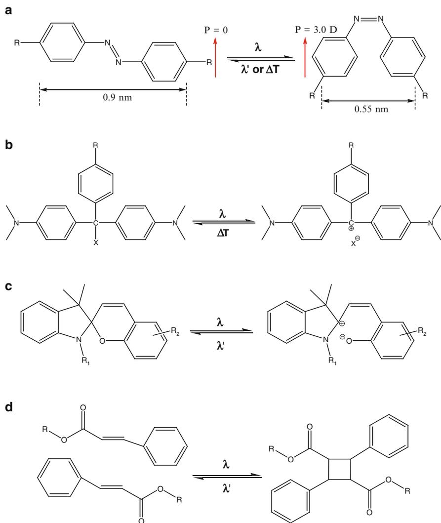
**Fig. 12** Examples of chromophores that display photochemically-induced transitions. **(a)** Reversible *trans* (left) and *cis* (right) photo-isomerization of azobenzene. **(b)** Dissociation of triphenylmethane leucoderivatives into an ion pair under ultraviolet irradiation. **(c)** Reversible photo-isomerization of spirobenzopyran derivatives. **(d)** Reversible photodimerization of cinnamoyl group
