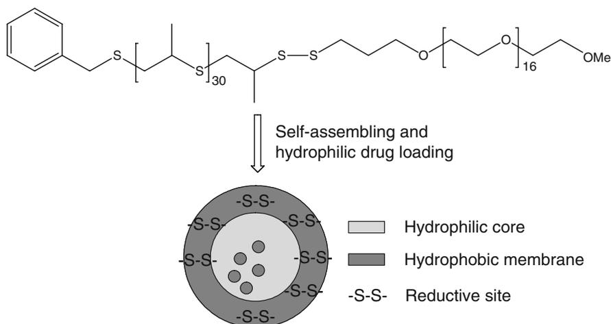
**Fig. 2** Polymersomes formed from the block copolymer, PEG<sub>17</sub>-SS-PPS<sub>30</sub>, where the hydrophilic poly(ethylene glycol) (PEG) and the hydrophobic poly(propylene sulfide) (PPS) are connected with a reductive disulfide group. (Reproduced from ref. Cerritelli et al. 2007)
