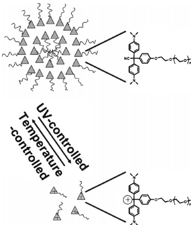
**Fig. 16** Schematic illustration of vesicles made from PEG and malachite green and their disassembly under UV illumination. (Reproduced from ref. Jiang et al. 2007b)
