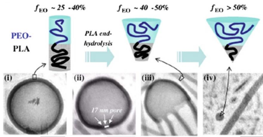
**Fig. 1** Representative time series showing the breakdown structures formed as PEG-*b*-PLA polymersomes transform from vesicles to worm-like micelles. The scale bars in the cryo-TEM images are 100 nm. (Reproduced from ref. Ahmed et al. 2006)
