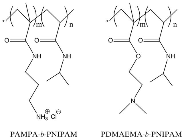
**Fig. 9** Hydrophilic-hydrophilic block copolymers with a temperature responsive block PNIPAM
