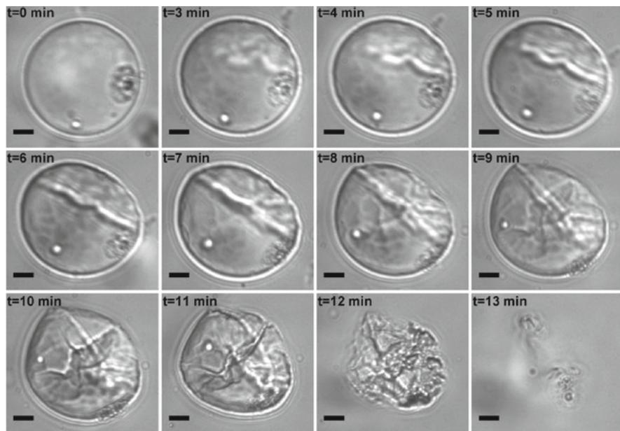
**Fig. 23** Bright-field microscope images showing the shrinkage and breakage of a PEG(5,000)-*b*-PLA(5,000) polymersome after an osmotic shock. As a result of water expulsion from its inside, the polymersome shrinks and buckles. Scale bar is 10  $\mu\text{m}$ . (Reproduced from Shum et al. 2008)
