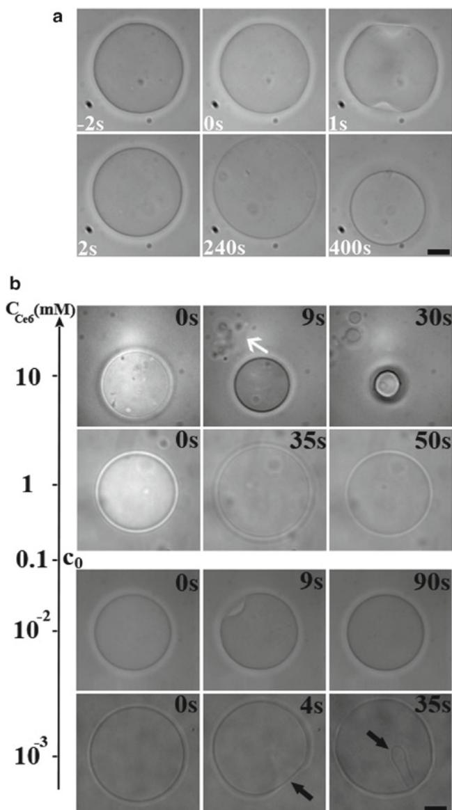
**Fig. 20** (a) Video sequence showing the morphological changes of Ce6-loaded PEO-*b*-PBD polymersomes under UV exposure. The bulk concentration of Ce6 is  $c_0 = 0.1$  mM. Irradiation starts at time  $t = 0$ . Scale bar =  $5 \mu\text{m}$ . (b) Representative UV-induced morphological changes of Ce6-loaded PEO-*b*-PBD polymersomes for different bulk concentrations of Ce6. The black arrows show the formation of membrane invaginations during UV illumination. Scale bar =  $5 \mu\text{m}$
