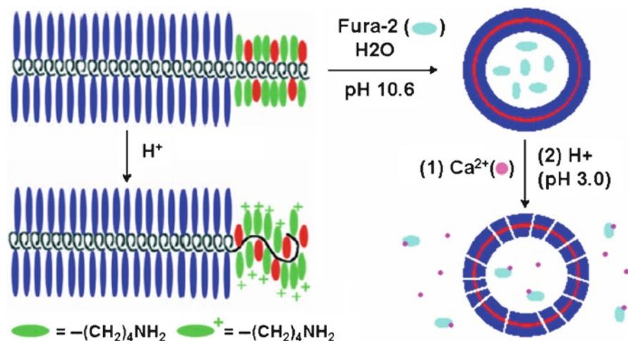
**Fig. 7** pH-responsive polymer vesicles formed from PELys-*b*-P(Leu<sub>0.3</sub>-*co*-Lys<sub>0.7</sub>)<sub>40</sub>. When the pH was lowered by addition of HCl, the release of entrapped Fura-2 dye took place within seconds. (Reproduced from ref. Bellomo et al. 2004)
