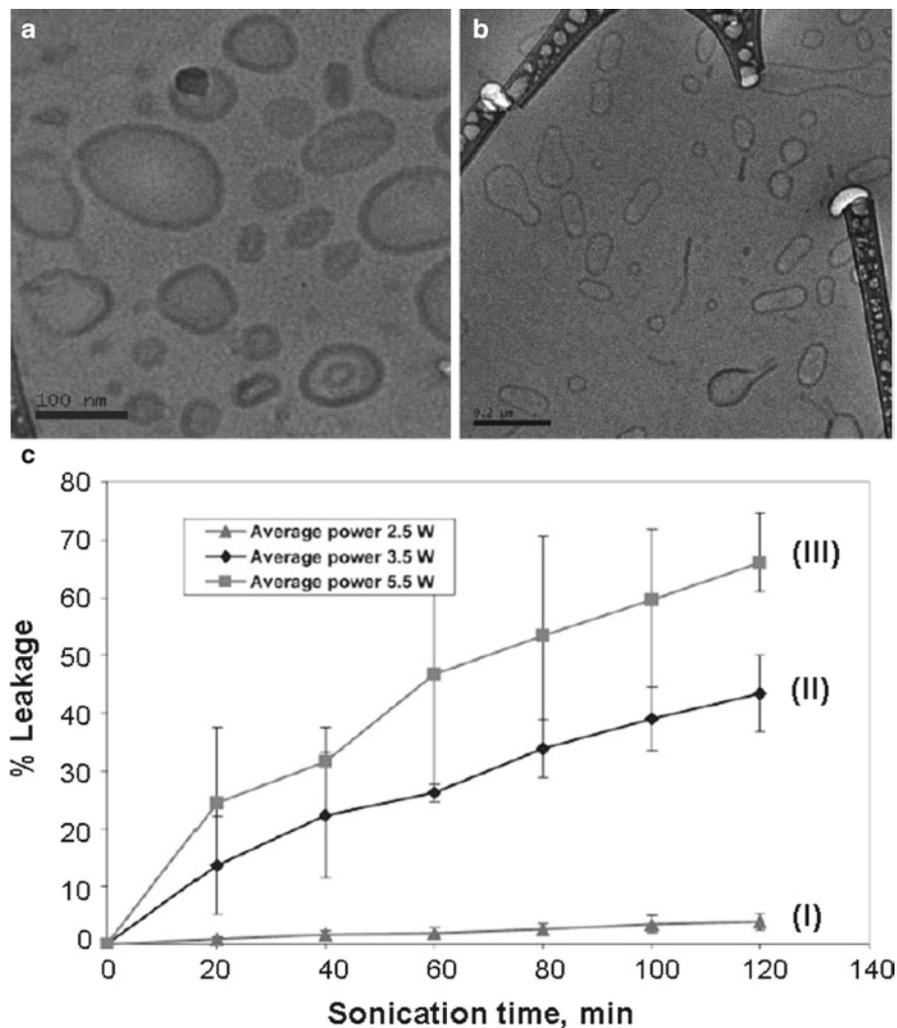
**Fig. 24** Cryo-TEM images of polymersomes (a) before and (b) after sonication. Scale bar= 100 nm in (a) and 200 nm in (b). Percentage of ANTS (8-Aminonaphthalene-1, 3, 6-trisulfonic acid, disodium salt) release as a function of time where the average sonication power during sonication cycles as recorded on sonic dismembrator dial was (I) 2.5 W, (II) 3.5 W, and (III) 5.5 W. (Reproduced from Pangu et al. 2010)
