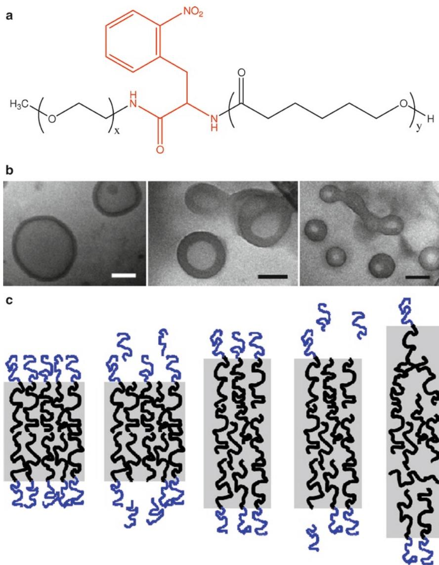
**Fig. 17** (a) Chemical structure of 2NPA linked PEG-*b*-PCL. (b) Cryo-TEM images of 2NPA polymersomes (*left to right*) before, during and after 6 h of UV exposure. Scale bars = 100 nm. (c) Schematic representation of membrane structures to explain the Cryo-TEM images. (Reproduced from Katz et al. 2010)
